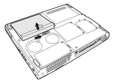
Removing the battery pack
